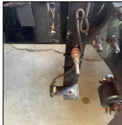
Figure 8: Ground Temp. Sensor
